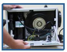
4. At this point, you can begin removing the screws on the cabinet. Start by removing the 3 screws on the drain hose side of the cabinet.
